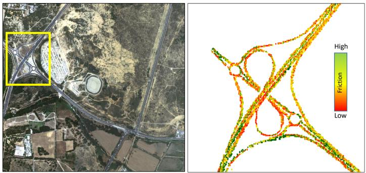
Figure 3: RGB image from HyMap sensor (left); derived friction coefficient vector point layer (right)
